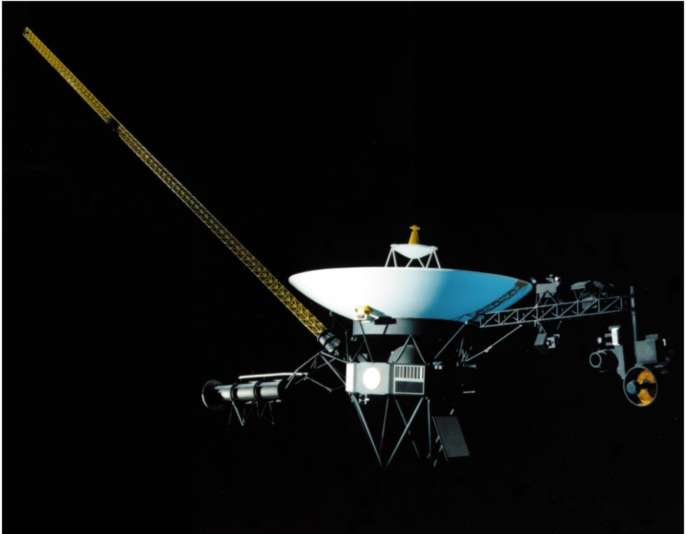
Figure 1. The Voyager spacecraft. In many ways, Voyager represents the “typical” planetary-science mission. Laden with a variety of instruments to study its targets in different wavelengths, it was sent to the outer planets on a flyby trajectory. Other missions combine landers, orbiters, and probes.
